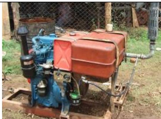
*The Feidong diesel engine, modified to run on PPO, with heat exchange in the exhaust; ready to be connected with an alternator for an endurance test.*
