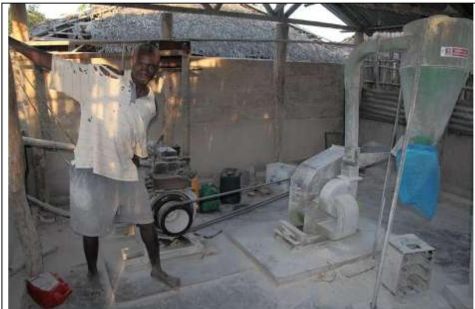
*Operator of maize mill with Feidong diesel engine*
