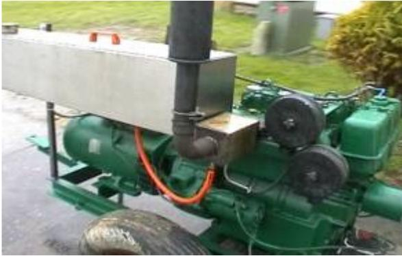
*Illustration 5: Heat exchanger and tank view.*
