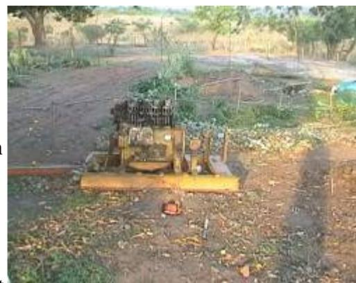
Illustration 10: Deutz engine stripped: fuel tank, oil cooler and mounting skid used
